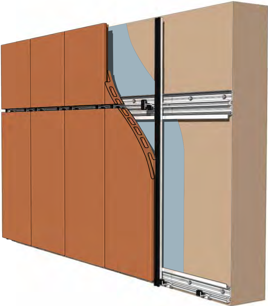
TERRACLAD™ SYSTEM DIAGRAM HORIZONTAL TRACK
