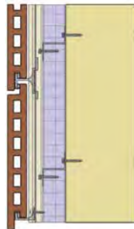
TERRACLAD™ SYSTEM SECTION DIAGRAM TOP - FLANGED TRACK BOTTOM - STANDARD TRACK
